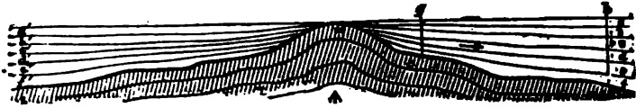
Fig. 6.—Ideal section of strata thinning out against a ridge. a , Upper Chalk; b , Lower Chalk; c , Upper Greensand; d , Gault; e , Lower Greensand; f , Neocomian beds; g , Old Wealden land.
